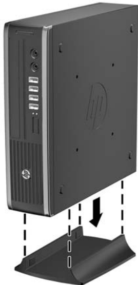
Figure 5-7 Placing the Computer on the Stand
